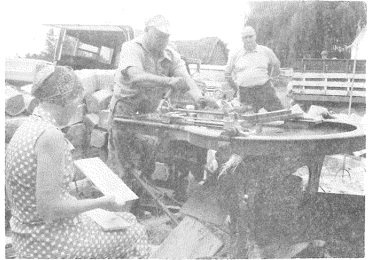
THERE WERE RELIEF OPERATORS --On the ancient shingle mill Saturday, relieving Lynn Mix, who brought the mill up from Hastings for the three-day job of providing cedar shingles fresh from cedar trees, for the roof of the Sherman City Church.
